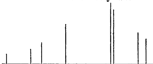
FIG. 8. Experimental and theoretical spectra of the -\text{CH}_2\text{OH} protons in benzyl alcohol. The experimental trace was observed with a solution of benzyl alcohol in acetone at mole fraction 0.5, room temperature, and 40 Mc./sec.
